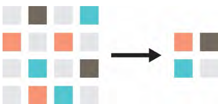
FIGURE 4. Deduplication—the process of removing data blocks, which are exact duplicates
